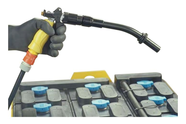
Simply connect the Watering Gun to a standard water hose or a Deionizer, put the tip of the gun into the cell and squeeze the ergonomic trigger. The mechanism will automatically shut off at exactly the right electrolyte level. The reliable PS Watering Gun speeds up battery watering, improves filling accuracy, and improves operator safety.
